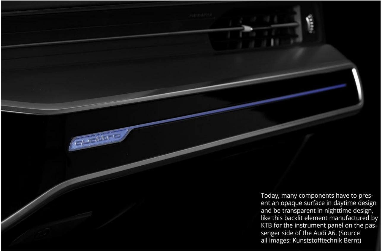
Today, many components have to present an opaque surface in daytime design and be transparent in nighttime design, like this backlit element manufactured by KTB for the instrument panel on the passenger side of the Audi A6. (Source all images: Kunststofftechnik Bernt)
